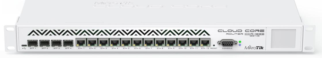
CCR1036-12G-4S is an industrial grade router with cutting edge 36 core CPU! Unprecedented power and unbeatable performance - this is our new flagship device, the Cloud Core Router (CCR1036). If you need many millions of packets per second - Cloud Core Router with 36 cores is your best choice.
